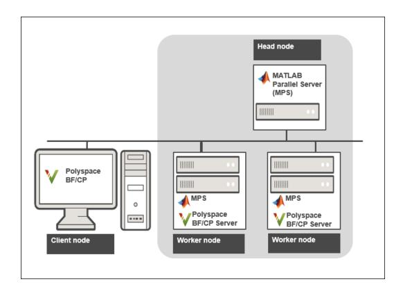
In the simplest remote analysis configuration, the same computer can serve as the head node and worker node. Note that you can run one Polyspace analysis on one worker only. You cannot distribute the analysis over multiple workers. Only if you submit more than one analysis job, you can distribute the jobs over multiple workers.
